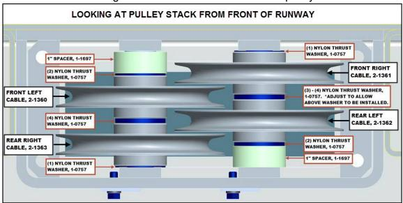
• Install rear right cable 2-1363 around the lower pulley.
