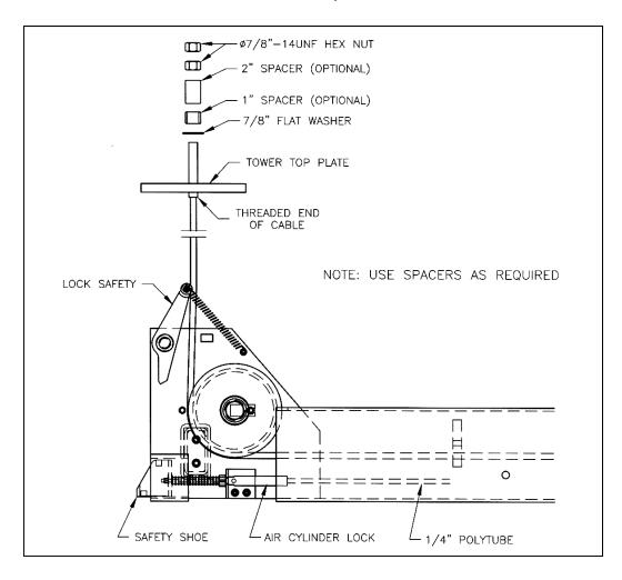
Figure 18. Cable routing diagram
