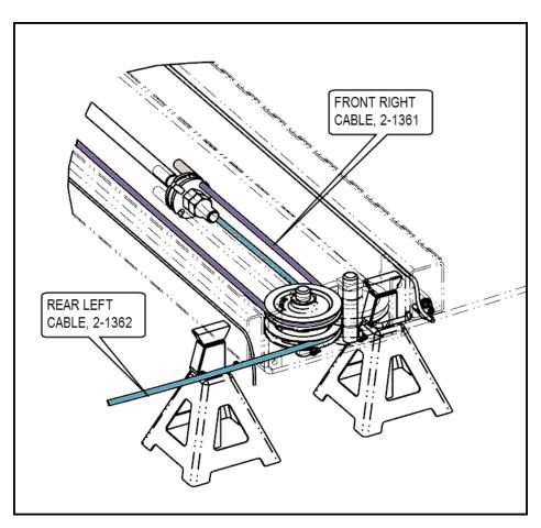
Figure 10. Front Right and Rear Left Cable Installed at Rear
