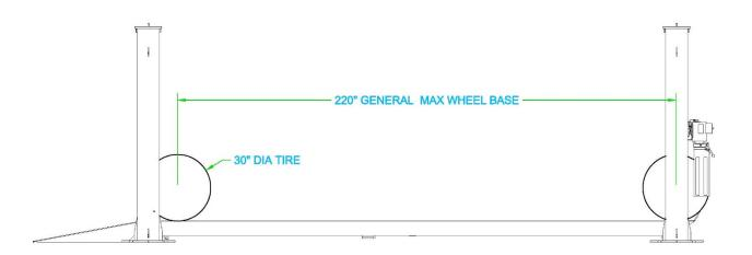
Figure 2 – Service & Alignment Wheelbase Specifications
