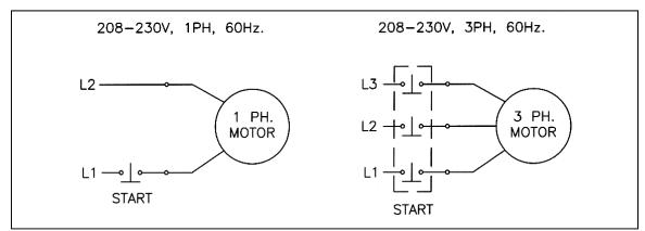
Figure 24. Electrical diagram for 230V/1 ph
