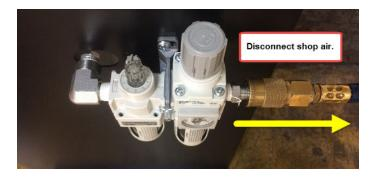
2. Using a slotted screwdriver or an Allen key, remove the filler cap from the top of the FRL.
