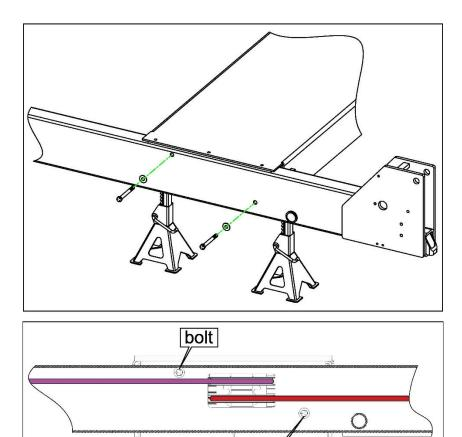
Figure 15. Fastening Crossmember to Deck
