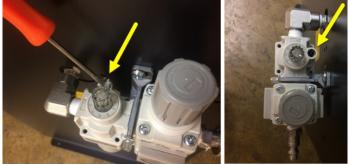
3. Fill FRL using Snap-On AirOil #IM6 or equivalent. Oil to be filled to the MAX line marked on reservoir. If unit does not have MAX line mark, reservoir should be 80% full.
