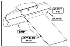
Figure 34: Approach Ramp Install
