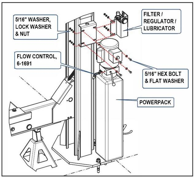
Figure 19. Power pack Install
