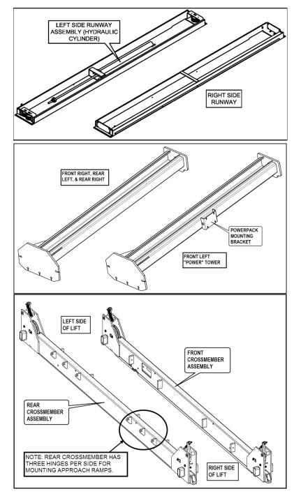
Figure 5. Component Identification
