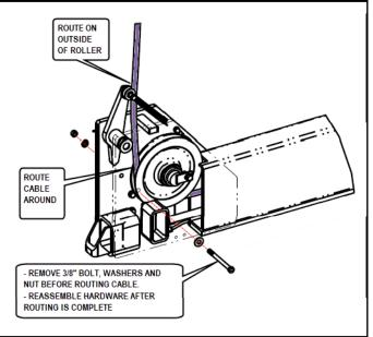
**NOTE:** Ensure retaining bolt is installed behind cable, not between cable and pulley.
