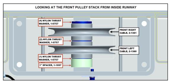
11. Use **Figure 11** as reference during the front pulley stack and cable assembly.
