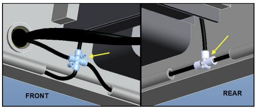
Figure 22. Air Connections
