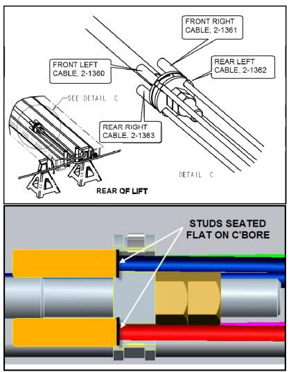
Figure 7. Cable Flange and Cable Assembly
