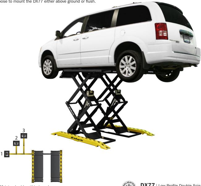
60" (standard length) air and hydraulic hoses allow three ergonomic, recommended power console placement options.
