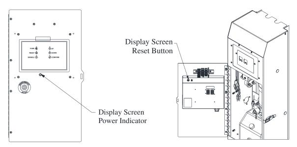
Figure 3. Control Panel Indicator Light and Display Screen Reset Button Locations
