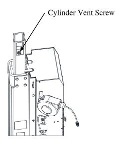
Figure 7: Cylinder Vent Screw
