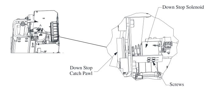
Figure 10. Down Stop Solenoid
