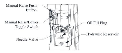
Figure 6. Manual Control Components
