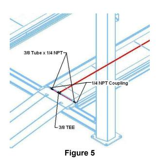
12. Route the 3/8" tube from the 3/8" tee in the passenger side front crossbeam to the 3/8" tee in the front drivers side runway as shown in Fig 6. Connect the 3/8" tube x 1/4" MNPT fitting to the 1/4" NPT coupling welded in the runway.
