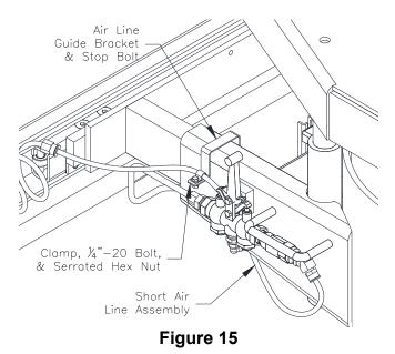
21. Remove Side Member Stop Bolt on the back side of the Jack arm. Install Air Line Guide Bracket and replace bolt. If necessary, adjust both the stop bolts on that end of the jack until both bolts can be tightened down.
