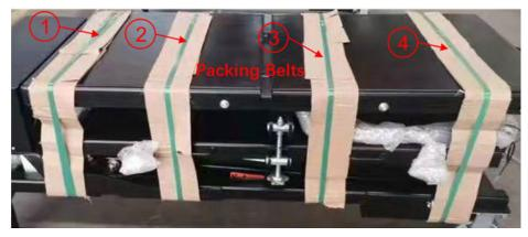
Fig.7.1.2 Packing Belts Position
