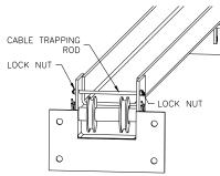
Fig. 5-Cable Trapping
