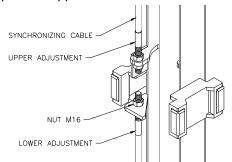
Fig. 6 - Synchronizing Cables
