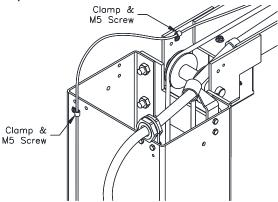
Fig. 10 - Lock Cable Routing
